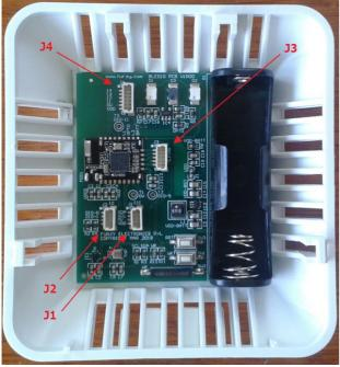
The BLE010 PCB has the option to fit 3 connectors for other IO and sensor connections (see the data sheets and case studies for the BLE010 with external sensors, refer to the schematic for details on pinouts and connections to the CC2640S1)
